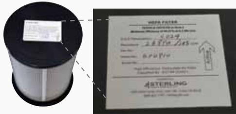
The HEPA filter is individually tested and certified to be 99.97% efficient at .3 microns according to IEST-RP-CC001 test requirement.
